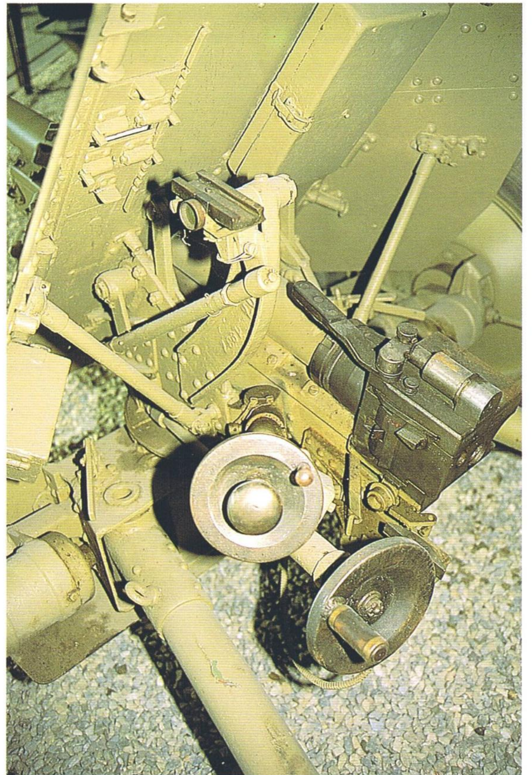
Fig.7 The aiming sight support arm from the other side (which differs from earlier PAK 37's) and both handwheels for azimuth and elevation adjustment of the gun. The top wheel elevates the gun barrel from -8^{\circ} to +25^{\circ} while the bottom wheel swivels the barrel over a 60^{\circ} arc of fire.
