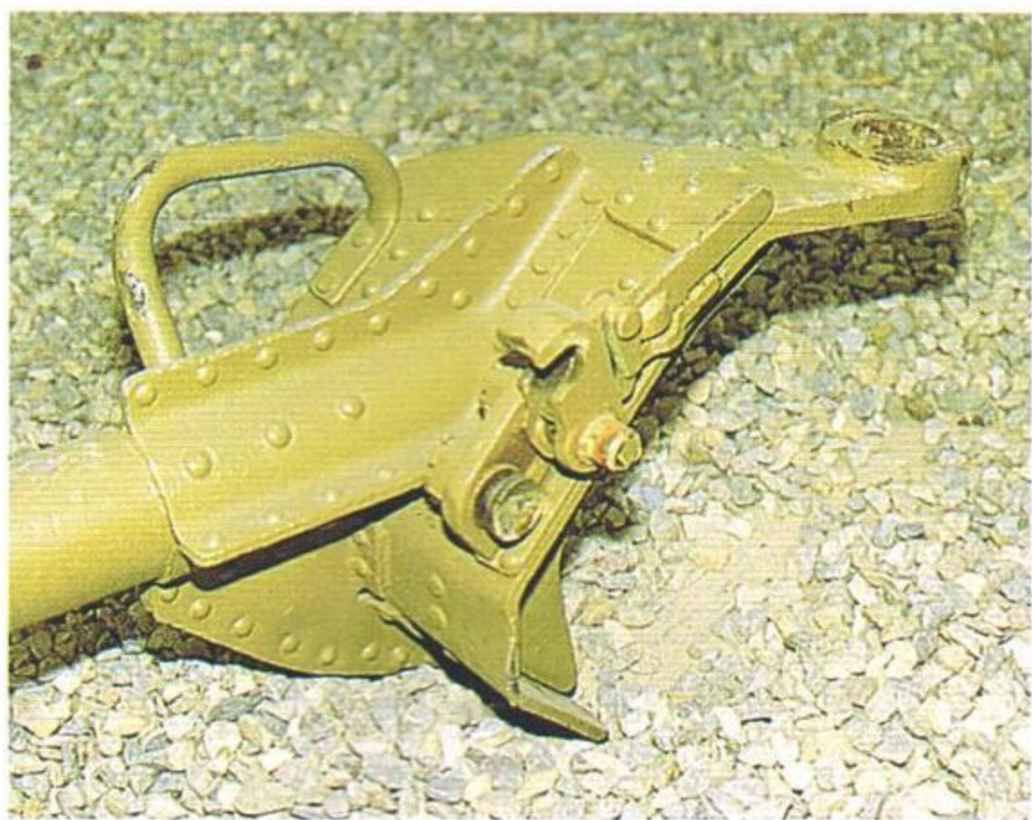
Fig.12&13 Two spade halves feature two massive handholds on the side which allow handpulling the gun. When transported over long distances the spade halves are locked together and hooked up behind a Kettenkrad.
