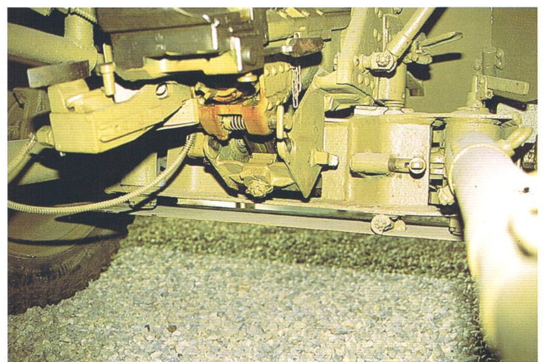
Fig.11 A gun assembly travel lock is mounted to the lower platform on the right side of the gun support frame. Also note the locking lever of the side arms at right.
