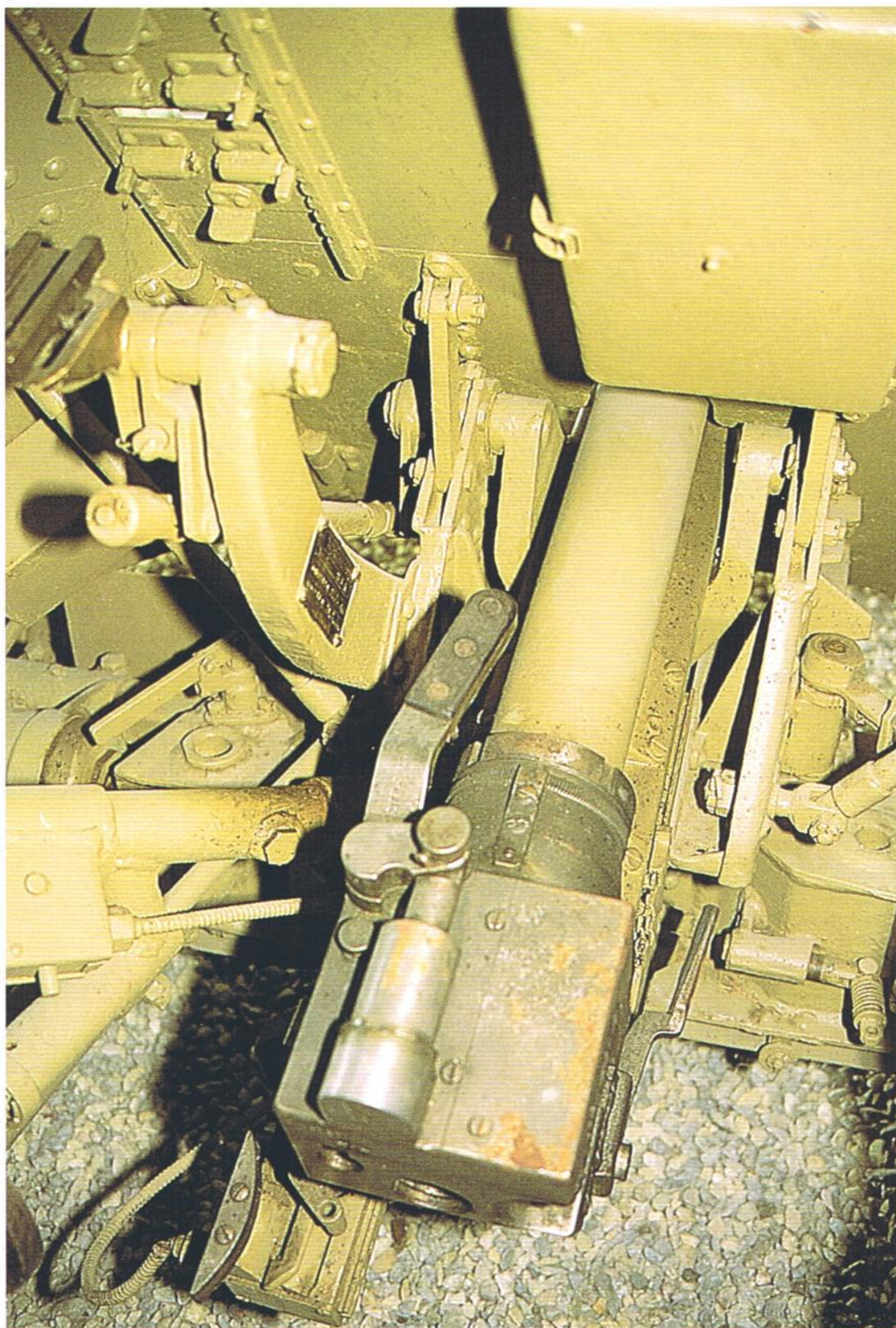
Fig.10 The complete gun assembly is hooked up inside two side-mounted supports which also serve as a main protective shield attachment. Note the breech block cocking lever.
